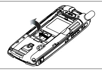
Insert USIM card into tray (notch in upper right corner, gold plate down).
