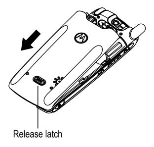
2 Slide USIM card door to the left and lift open.
