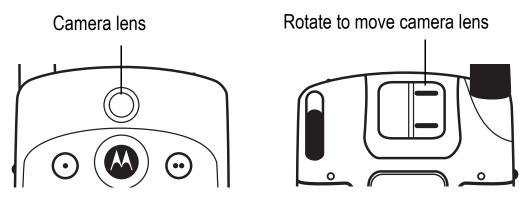
**Note:** To protect the lens when not using the camera, position it so that it faces the top of the handset.
