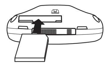
If you need to remove the memory card, push it into the slot until it unlocks. Then slide it out.
